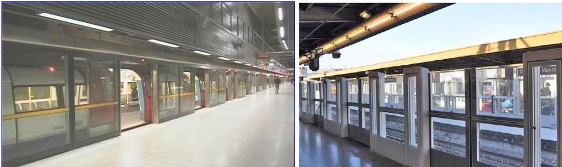
*Platform Screen Doors can be designed for full coverage in underground stations, and partial coverage for surface and above-ground stations. (Source: Wikimedia Commons)*
