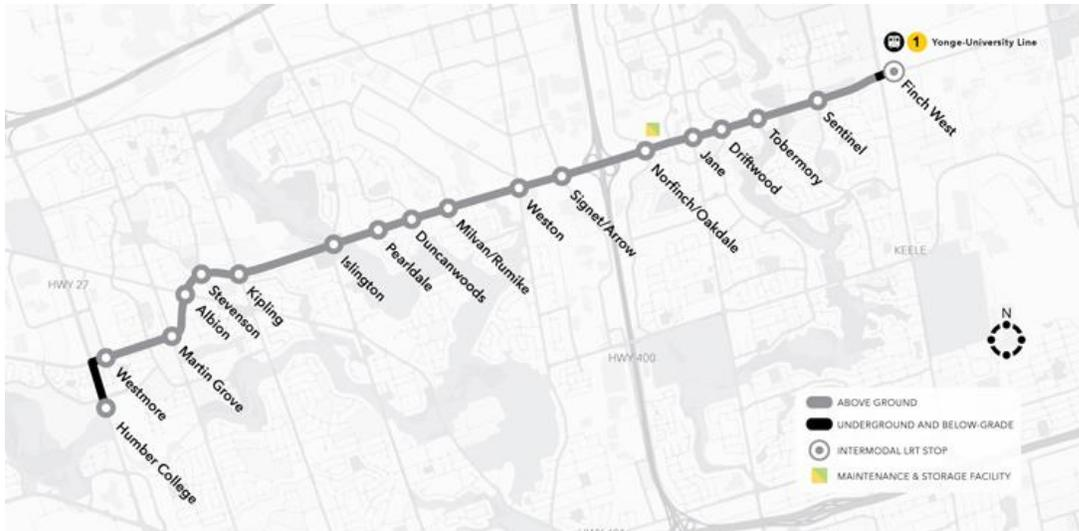
The Finch LRT line will run down the centre of Finch Avenue in a dedicated right-of-way, with an underground section at Keele Street as it enters Finch West subway station at the eastern terminus. The line will tunnel under the intersection of Finch Avenue and Highway 27, and emerge to an open cut section along Highway 27 to its western terminus just south of Humber College Boulevard.
