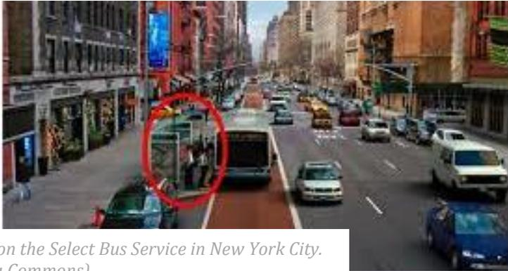
This type of treatment has a cost of approximately \$2 million per kilometre, a very low cost by any standard, as it simply involves painting red bus lanes that have been created by dedicating existing vehicle travel lanes, or by reducing on-street parking. This has
